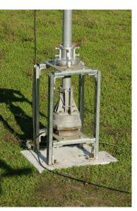
All this was tilted over to Clark's driveway where it rested on a step ladder and provided the necessary elevation to attach the Yagi antenna. Once the U-bolts where tight, the coax was attached with a clearance loop that would allow unhindered rotation.
